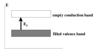
Fig. 11.4.4 The energy diagram of an insulator.
