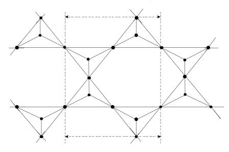
Fig. 7.11 Structure of the  $Si_4O_{10}^{4-}$  ion.
