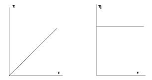
Fig. 9.18 Newtonian flow behaviour.
