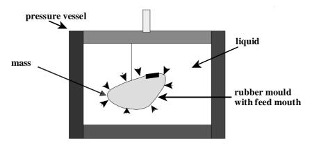
Fig. 9.15 Compressing powders isostatically.
