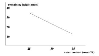
Fig. 9.11 Graphic representation of Pfefferkorn measurements.
