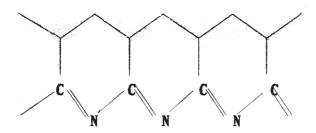
Fig. 14.5 PAN chain after initial heating.
