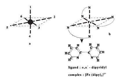
Fig. 13.1 The general structure of an octahedral complex (a) and the structure of a red-coloured iron complex (b).
