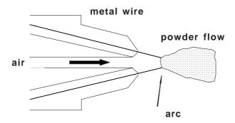
Fig. 11.7.10 Arc spraying.
