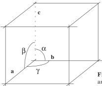
**Fig. 4.6** A three-dimensional point lattice and an elementary cell from the lattice.
