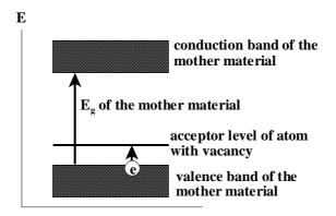
Fig. 11.4.10 Energy diagram of a p-type semiconductor.
