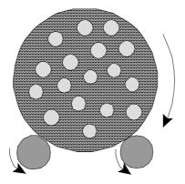
Fig. 9.6 Mill with ceramic balls.
