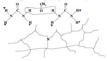
Fig. 10.3 The formation and structure of a urea-formaldehyde resin (UF), a thermosetting resin.
