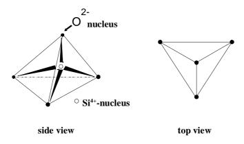
Fig. 7.8 Structure of the SiO<sub>4</sub> tetrahedron.
