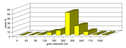
Fig.9.3 Histogram of a grain size distribution.
