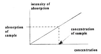
Fig. 13.3 Calibration line of a spectrophotometric analysis.
