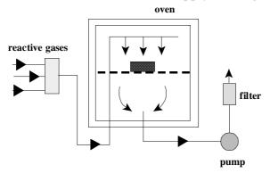
Fig. 11.7.9 Schematic representation of a CVD unit.
