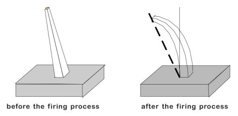
Fig. 11.3.1 The application of a Seger cone.
