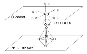
$\textbf{Fig. 8.7} \quad \text{The linking of an O- and a T-sheet}.$
