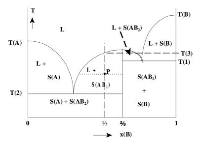
Fig. 6.9 T,x diagram of a binary system with a congruently melting compound.
