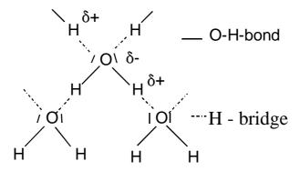
Fig. 3.12 Hydrogen bridges between water molecules.
