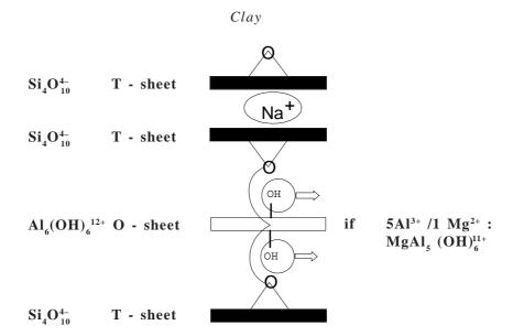
Fig. 8.8 Structure of the clay mineral montmorillonite.
