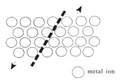
Fig. 10.5 Parts of the crystal lattice of a metal move along a crystal plane under the influence of external forces.
