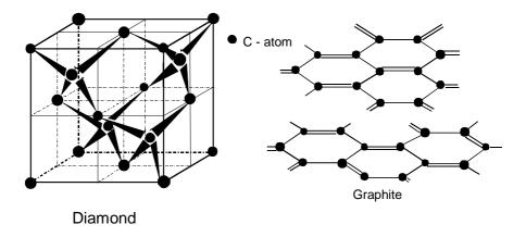
Fig. 3.13 Crystal structures of diamond and graphite.
