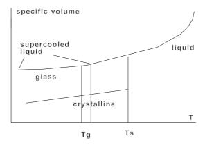
Fig. 11.1.2 Specific volume versus temperature for a glass.
