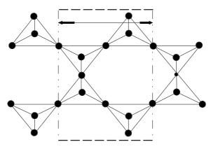
Fig. 8.5 The structure of a silicate ion in a clay mineral.
