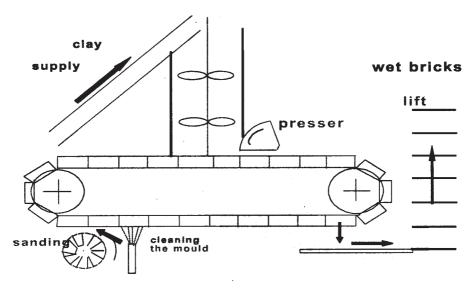
Fig.11.2.2 Press moulding. (source: Koninklijk Verbond van Nederlandse Baksteenfabrikanten [Eng.:Royal Association of Dutch Brick Manufacturers])
