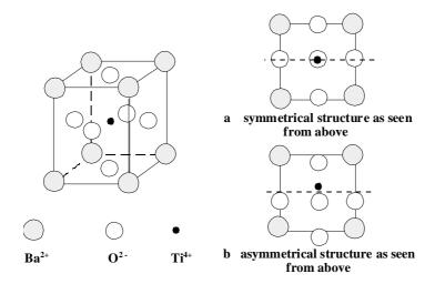
Fig. 11.4.25 Unit cell of barium titanate.
