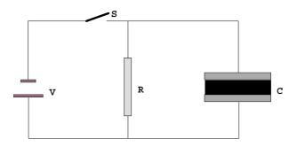
Fig. 11.4.20 Circuit for the discharge of a capacitor.
