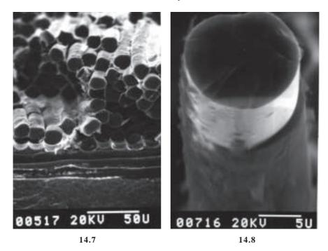
**14.6** As in 14.3, but during two hours at 1750 °C, not coated. **14.7** SEM micrograph of BN-coated Hi-Nicalon fiber for use as a reinforcement of a SiC/SiC-composite. (Source: Nippon Carbon Co Ltd Japan).
