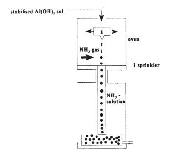
Fig. 11.7.7 Production of microspheres according to the BRACE-method.
