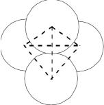
Fig. 4.2 Pyramid-formation by spheres in a close-packed structure.
