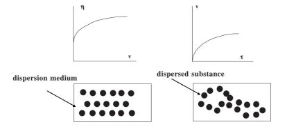
Fig. 9.20 Dilatant flow behaviour.
