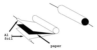
Fig. 11.4.22 The construction of a cylindrical capacitor.
