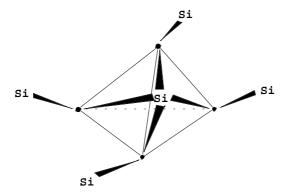
Fig. 7.12 Structure of the three-dimensional silicate anion.
