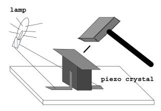
**Fig. 11.4.27** Test rig for a demonstration of the piezoelectric effect. (Source: Crystals and Crystal Growing, Doubleday & Company).
