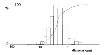
Fig. 13.5 Histogram of the mass percentage of particles as a function of the particle diameter and the accompanying cumulative curve.
