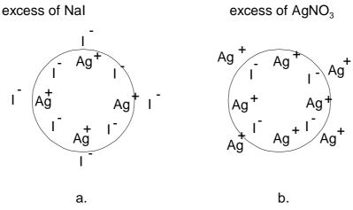
Fig. 5.7 Schematic representation of a negatively (a) and a positively (b) charged silver iodide sol.
