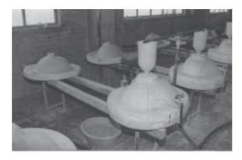
Pouring clay suspension in a mould for producing a wash basin at Sphinx sanitary (by J.Aarsen).
