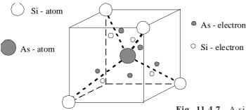
**Fig. 11.4.7** A silicon crystal doped with arsenic atoms.
