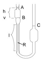
Fig. 5.10 Ostwald viscometer.
