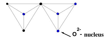
Fig. 7.9 Structure of the  $Si_2O_7^{6-}$  anion.
