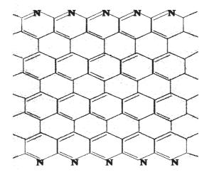
Fig. 14.7 Structure of a carbon fibre.
