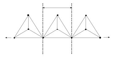
Fig. 7.10 Possible structure of a silicate chain.
