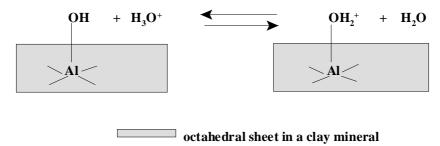
Fig. 9.16 A surface charge on a clay sheet.
