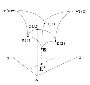
Fig. 6.11 Diagram of a ternary system with three binary eutectics and a ternary one.
