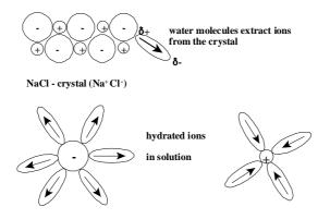
Fig. 3.11 Dissolving sodium chloride in water.
