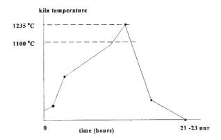
Fig. 11.1.11 Firing curve of sanitary ware.
