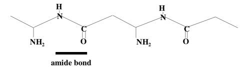
Fig. 3.23 Simple representation of a polyamide chain (both  $NH_2$  groups do not belong to the basic structure).
