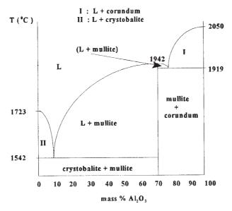
Fig. 11.3.3 Phase diagram of the system SiO<sub>2</sub> / Al<sub>2</sub>O<sub>3</sub>.
