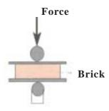
Fig. 11.2.3 Measuring the fracture strength of a brick.
