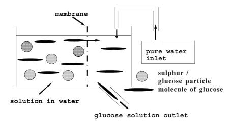
Fig. 5.5 Dialysis of a sulphur / glucose solution.
