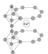
It is possible to draw the octahedron on the 8 - ring four times. The structure can be seen as the CsCl - structure with  $B_6$  - octahedrons instead of Cl - ions
