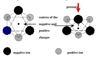
Fig. 11.4.26 Fictitious crystal unit of a piezocrystal, not subjected and subjected to pressure.
