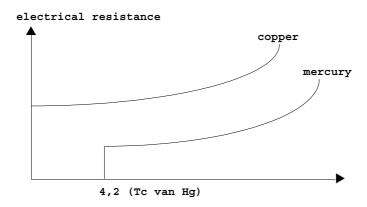
Fig. 11.4.11 Electrical resistance of copper and mercury as a function of temperature.
