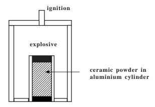
Fig.12.3 Simplified trial set-up for the explosive densification of a ceramic powder.
