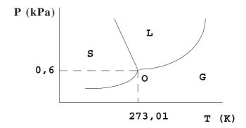
Fig. 6.5 P, T diagram of water.
