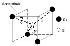
Fig. 11.4.9 Crystal lattice of germanium with doped boron atoms.
