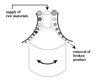
Fig. 9.5 Conical crusher.
