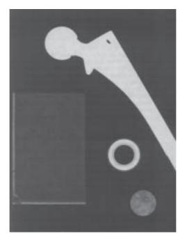
X-ray photograph of a hip joint, a rectangular piece of foam ceramics, a round glass reinforced with titanium fibers and a ring made of metal and ceramics (picture by J Bormans).
