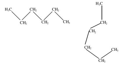
Fig. 3.15 Two conformations of the hexane molecule.
