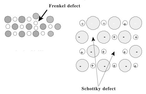
Fig. 4.8 Point defects.
