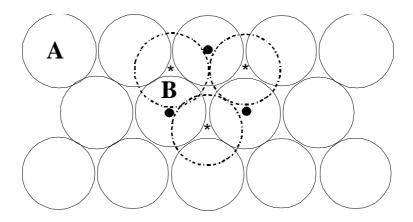
Fig. 4.4 An octahedral cavity in a close-packed structure.
