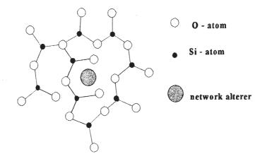
Fig. 11.1.5 Network alterers in quartz glass.
