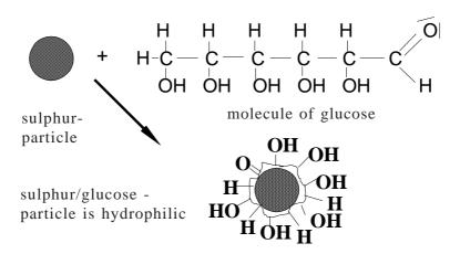
Fig. 5.4 A hydrophobic sulphur particle is made hydrophilic.
