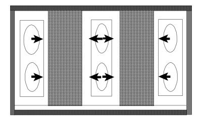
Fig. 9.24 Drying chamber for paving bricks.
