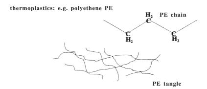
Fig. 10.2 The structure of polyethene (PE), a thermoplastic.
