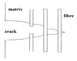
Fig. 14.9 Crack formation in a fibre-reinforced matrix.
