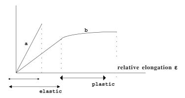
Fig. 9.29 Elongation diagram of a ceramic material (a) and a metal (b).
