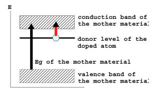
Fig. 11.4.8 Energy diagram of an *n*-type semiconductor.
