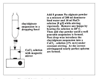
Fig. 11.7.8 Manufacturing clay microspheres.
