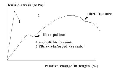
Fig. 14.10 Tensile stress as a function of the relative change in length of a non-reinforced (monolithic) and of a reinforced ceramic material.
