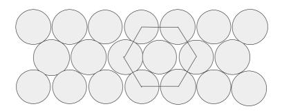
Fig. 4.1 Close-packed structure of spheres in a layer.
