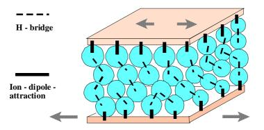
Fig. 9.9 The plastic behaviour of clay.
