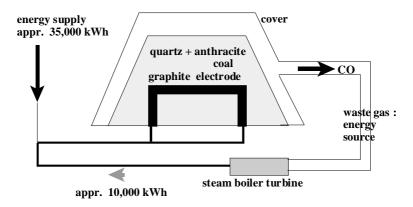
Fig.9.1 Synthesis of silicon carbide.
