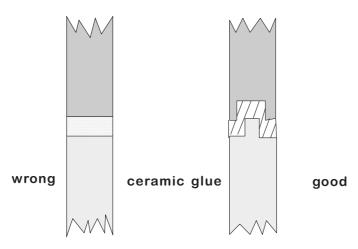
Fig. 11.7.2 Increasing the area of contact for applications at high temperatures.
