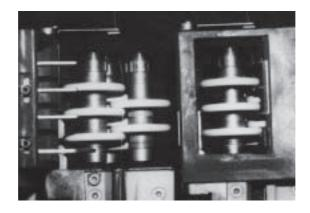
Ceramic friction discs in textile industry (Feldmühle, Germany)
