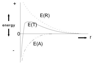
**Fig. 5.9** Representation of the interaction energy E(T) between two colloidal particles  $[E(R) = \text{repulsion energy} \quad E(A) = \text{attraction energy} \quad E(T) = E(R) + E(A), r = \text{distance between two particles}].$
