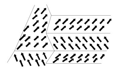
Fig. 11.5.2. Magnetic domains in a ferromagnetic material.
