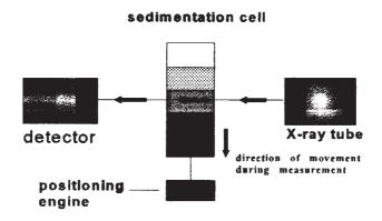
Fig.13.4 The principle of a Sedigraph.
