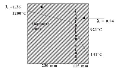
Fig. 11.3.2 The effect of insulation bricks.
