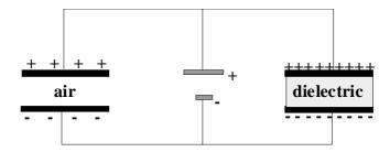
Fig. 11.4.18 Comparison of capacitors with and without dielectrics.
