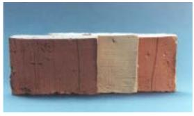
Different baking colours of bricks (by J.Aarsen).
