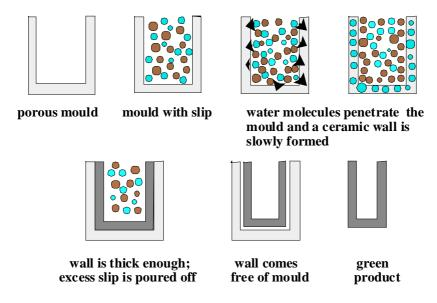
Fig. 9.21 Slip casting.
