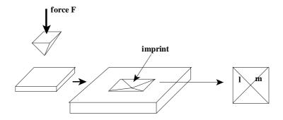
Fig. 9.28 Hardness measurement according to Vickers.
