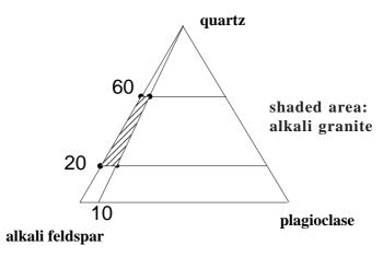
Fig. 8.2 Composition triangle of rocks containing the components quartz, alkali feldspar and plagioclase.
