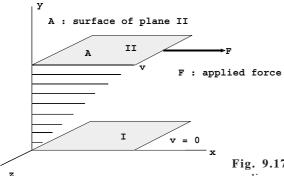
Fig. 9.17 Laminary flow in a liquid medium.
