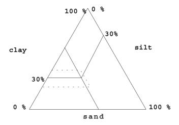
Fig. 8.1 Ternary compostion triangle for clay-containing soils.
