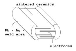
Fig. 11.4.23 A multi-layer capacitor.
