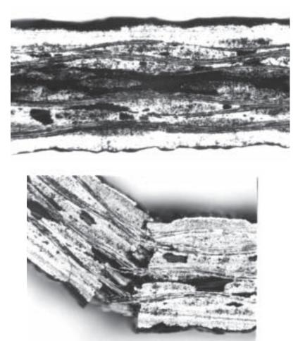
Photo 14.1 / 14.2 Optical micro-photograph of a  $SiC/SiC_f$  composite, made by means of CVI before and after a three point bending test (source: Ube Industries Co Ltd Japan).
