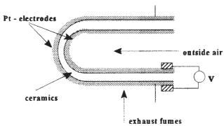
Fig. 11.7.4 Extremely schematic representation of the labda-probe.
