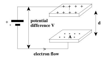
Fig. 11.4.17 Charging a capacitor.
