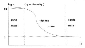
Fig. 11.1.10 Viscosity of a glaze as a function of temperature.
