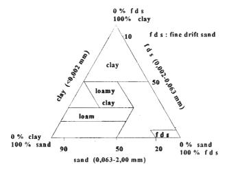
Fig. 11.2.1 Phase diagram of loam, clay and sand.
