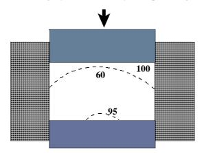
Fig. 9.14 Uniaxial compression of a powder (pressure variations are indicated in percentages of applied pressure).
