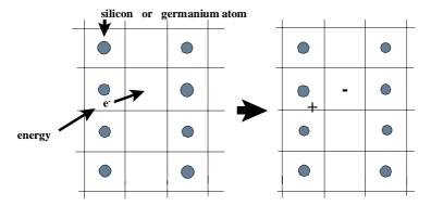
Fig. 11.4.6 Conduction in a silicon or germanium crystal.
